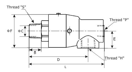
WS-Silicon carbide to carbon graphite mechanical seals.
