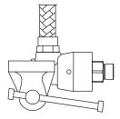
2. Always attach the hose before installing on the machine. Clamp rear of union in a bench vise.
