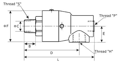
WS-Silicon carbide to carbon graphite mechanical seals.
